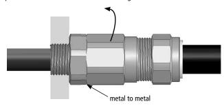
6. Only using finger pressure, tighten the outer seal nut assembly (8) until light resistance to tightening is met.
